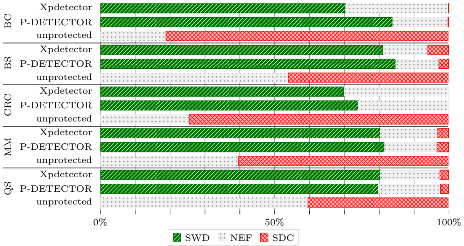
Figure A.6: The results of the single-bit DFE fault injection campaigns on the BC, BS, CRC, MM, and QS case studies protected with P-DETECTOR on the RV32I and RV32IXpdetector ISAs.
